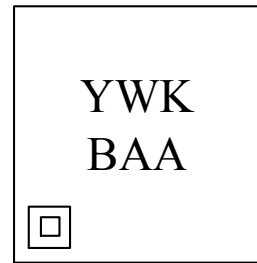
9 Bump WLCSP Marking (Top View)
